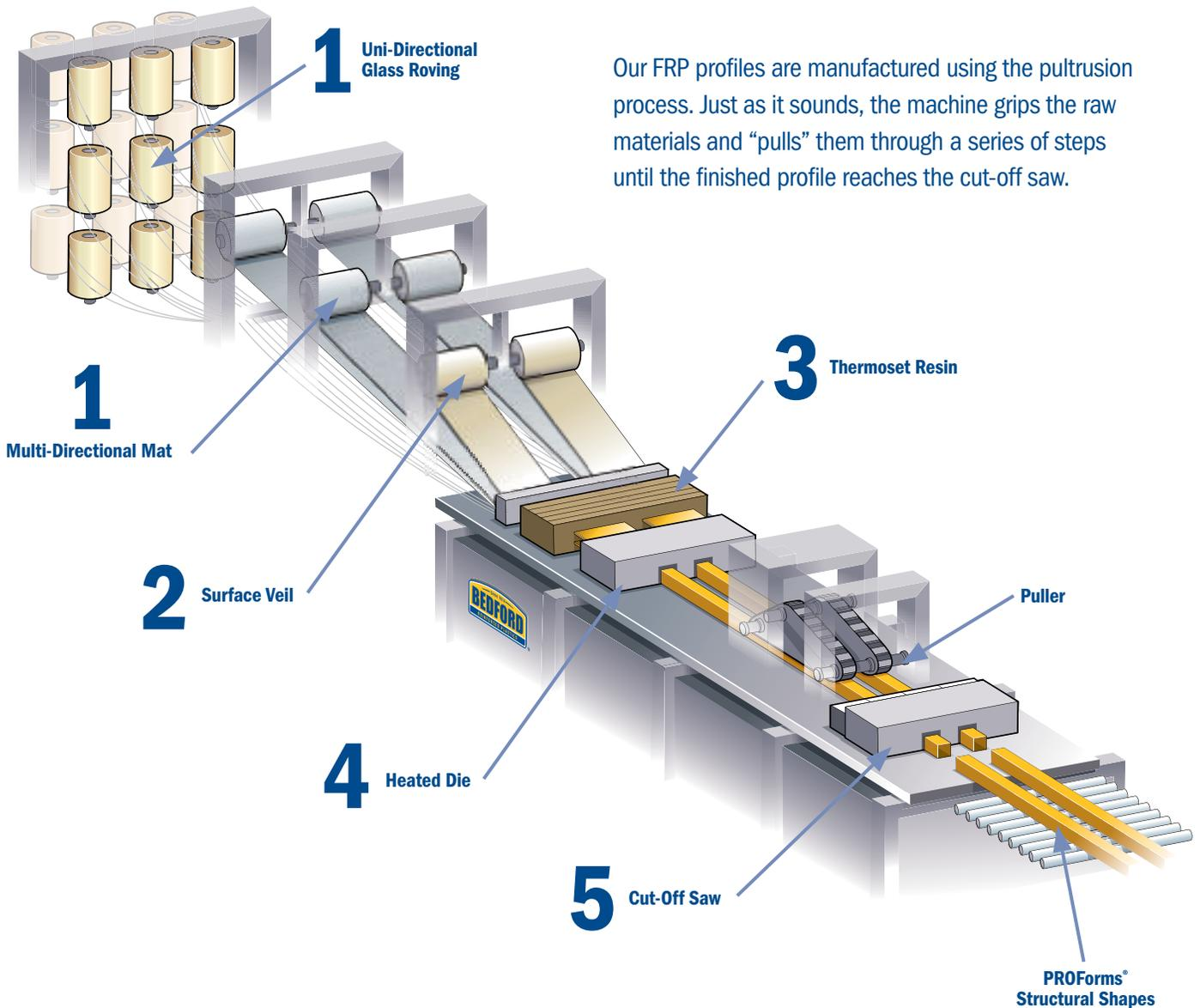
Our FRP profiles are manufactured using the pultrusion process. Just as it sounds, the machine grips the raw materials and “pulls” them through a series of steps until the finished profile reaches the cut-off saw.
